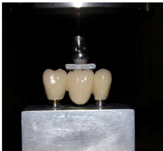
**Fig. 2:** Position of stainless steel ball and Teflon disk at loading point
