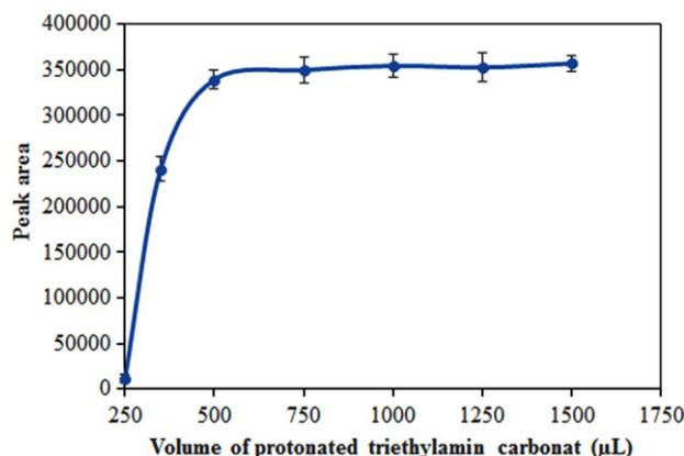
**FIGURE 2** Effect of the extractant volume (protonated triethylamine carbonate) on the extraction of PQ; Conditions: sample volume (10 mL; 100 µg/L of PQ), NaOH volume (2.0 mL (10 mol/L))
