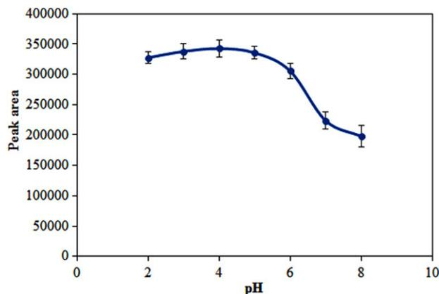
**FIGURE 1** Effect of pH on the extraction of PQ; Conditions: sample volume (10 mL; 100 µg/L of PQ), extractant volume (500 µL), NaOH volume (2.0 mL (10 mol/L))
