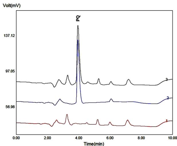
**FIGURE 3** HPLC–UV chromatograms of (1) urine blank sample after microextraction (Red) (2) standard solution of PQ (7 mg/L) (Blue), and (3) spiked urine sample by 100 µg/L of PQ after microextraction (Black)
