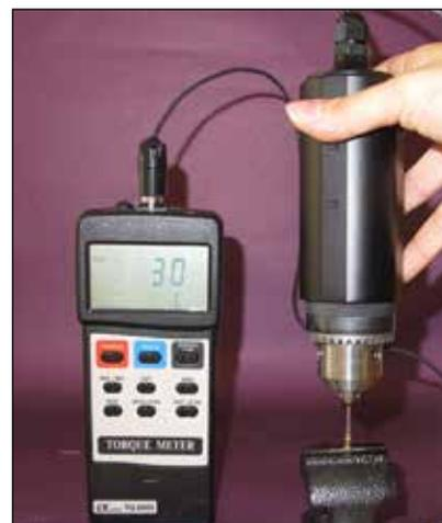
**Fig 3** Torque application with electronic torque meter.
