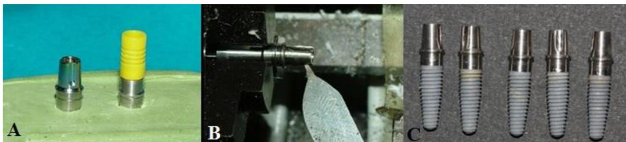
**Fig. 2:** Fabrication process of GoldAdapt samples, (A) wax up, (B) milling procedure, (C) GoldAdapt samples
