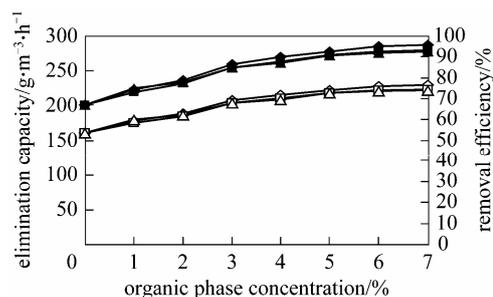
**Figure 2** Effect of various organic phase concentration on the bioreactor elimination capacity and removal efficiency for BTX
