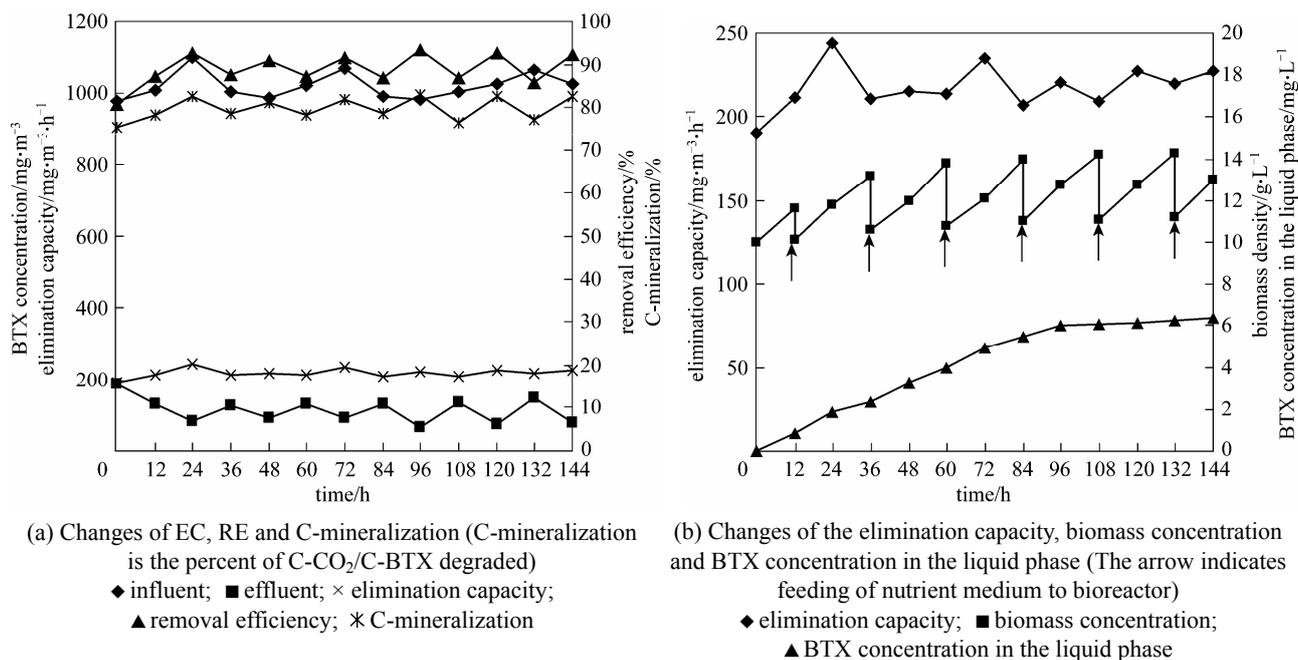
**Figure 7** The continuous operation of bioreactor
