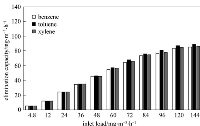
Figure 6 Elimination capacity of bioreactor for individual BTX versus different inlet loads
