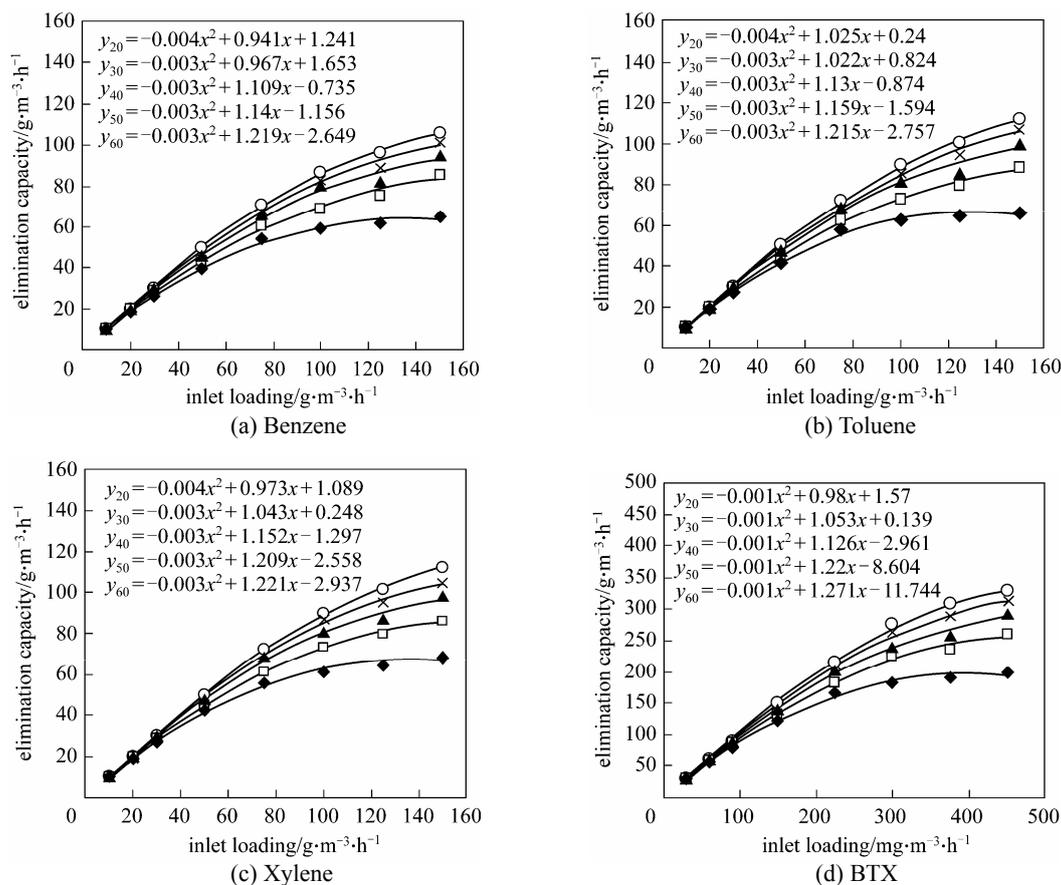
**Figure 3** Effect of oxygen content of inlet air to bioreactor on the elimination capacity of benzene, toluene, xylene and BTX (Experimental conditions:  $1 \text{ g}\cdot\text{m}^{-3}$  of inlet BTX concentration, 15 s of residence time,  $10 \text{ g}\cdot\text{L}^{-1}$  of biomass concentration)  $\blacklozenge$  20%;  $\square$  30%;  $\blacktriangle$  40%;  $\times$  50%;  $\circ$  60%
