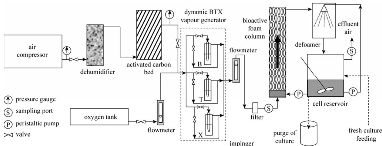
Figure 1 Schematic of the studied bioactive foamed emulsion reactor
