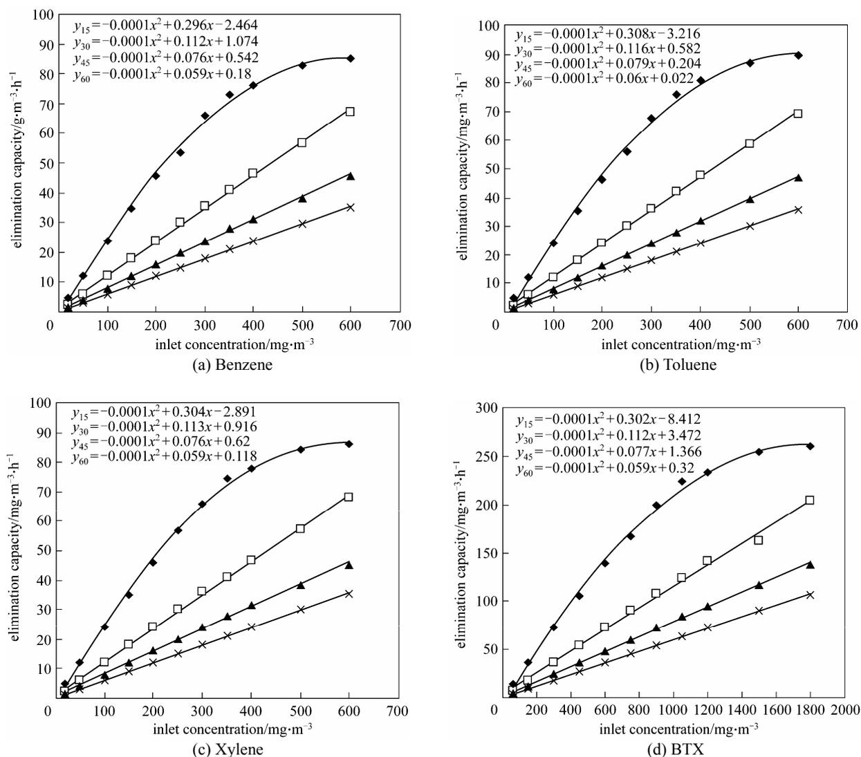
**Figure 4** Effect of gas residence time on the elimination capacity for benzene, toluene, xylene and BTX (Experimental conditions:  $10 \text{ g}\cdot\text{L}^{-1}$  of biomass concentration and 40% oxygen content at inlet gas stream)
