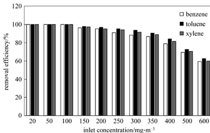
Figure 5 Removal efficiency of individual B, T, X compound for various inlet concentrations
