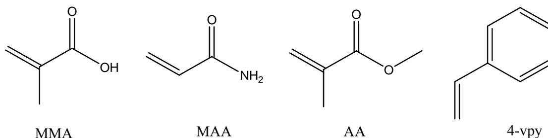
**Fig 2.** Chemical structures of the functional monomers used to polymer preparation
