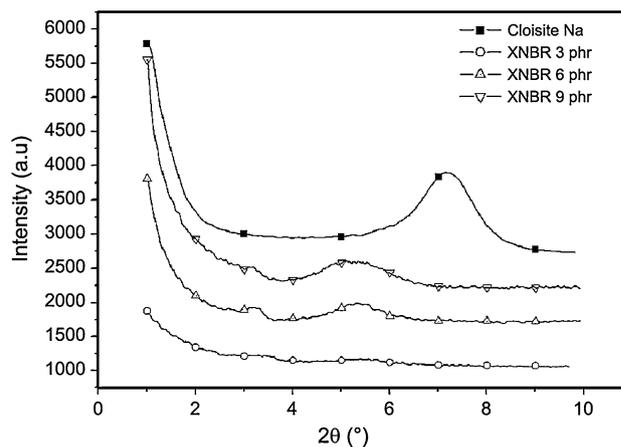
**Fig. 4** XRD diffractograms of Cloisite Na<sup>+</sup> and nanocomposite films having different amounts of nanoclay
