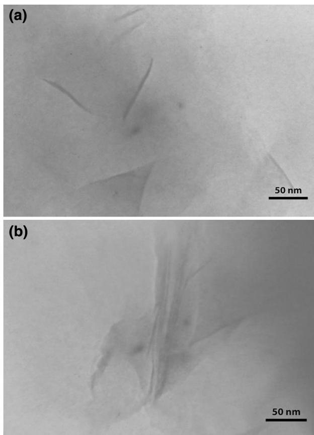
**Fig. 5** TEM images of the XNBR–clay nanocomposites at: **a** 3 (XNBR<sub>3</sub>) phr and **b** 9 (XNBR<sub>9</sub>) phr loading
