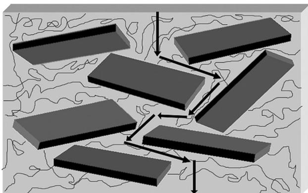
**Fig. 7** Schematic representation of how tortuous path can longer the traveled distance of solvent molecules through the nanocomposite
