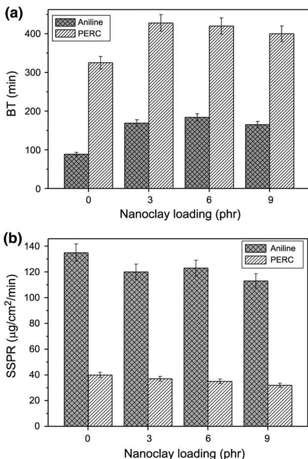
**Fig. 6** **a** Breakthrough time (BT) and **b** SSPR for selected solvent through XNBR–clay nanocomposites at different nanoclay loadings
