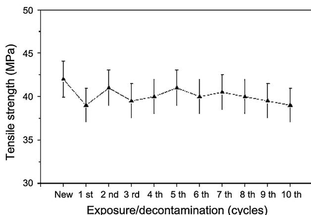
**Fig. 8** Change in tensile strength of XNBR<sub>3</sub> nanocomposite against aniline after exposure/decontamination cycles
