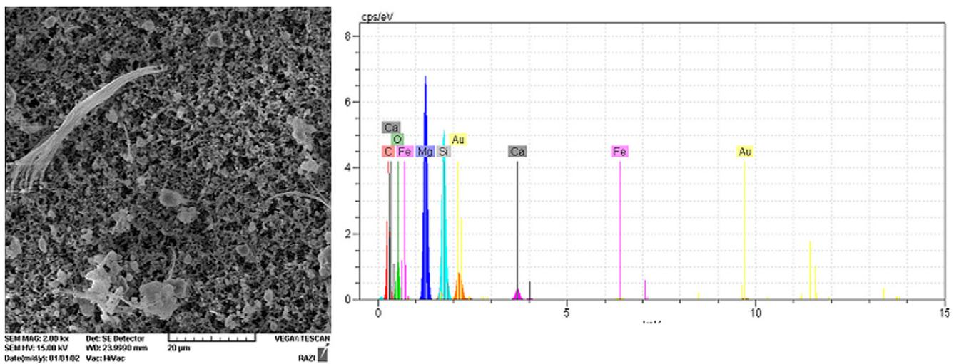
Fig. 4. SEM image and EDS spectrum of airborne chrysotile. Magnification, 2000×.
