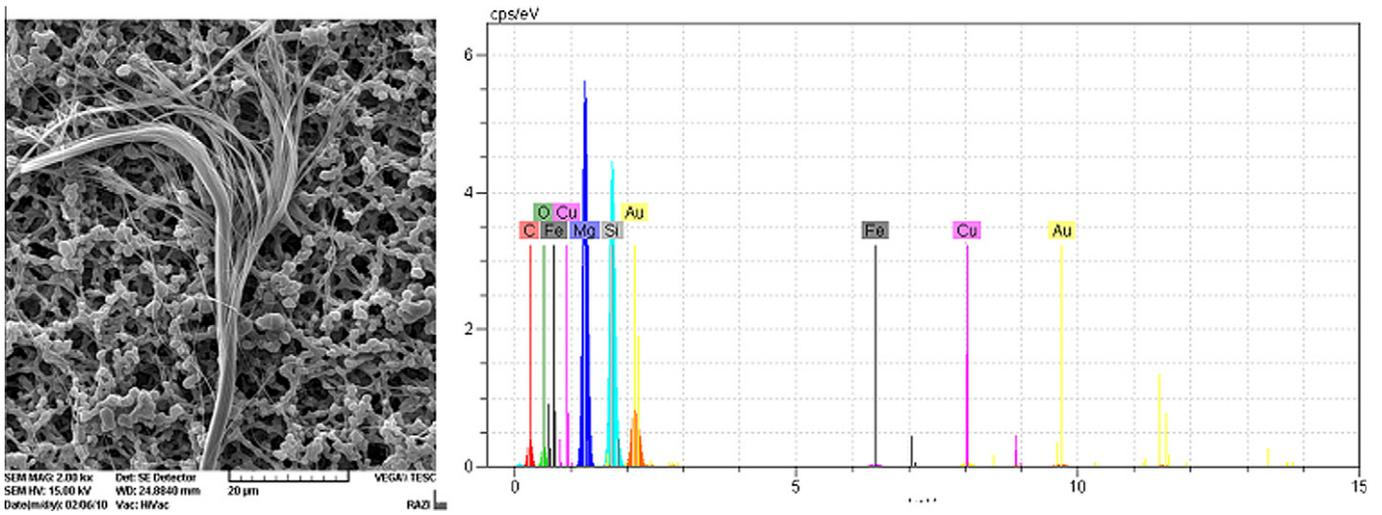
Fig. 3. SEM image and EDS spectrum of chrysotile (raw materials). Magnification, 2000×.
