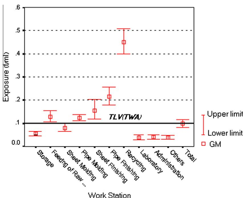
Fig. 1. Confidence interval of airborne fiber concentration (f/ml) in different workstations of an AC sheet and pipe manufacturing factory, as determined by PCM.
