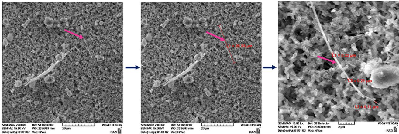
Fig. 5. Determination of fiber size by SEM. Magnification, 2000× & 10000×.
