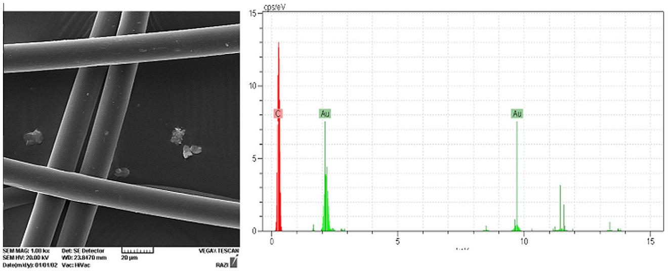
Fig. 2. SEM image and EDS spectrum of polypropylene fibers (raw materials). Magnification, 1000×.
