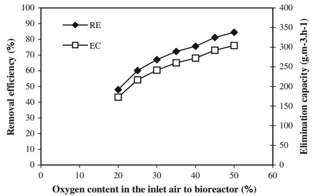
**Fig. 5** Effect of oxygen content in the inlet air to bioreactor on the removal efficiency and elimination capacity. Experimental conditions: 1.5 g m<sup>-3</sup> of inlet benzene concentration, 15 s of residence time, 15 g L<sup>-1</sup> of biomass concentration
