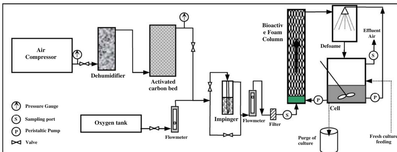
**Fig. 1** Schematic of the bioactive foamed emulsion reactor applied in this study
