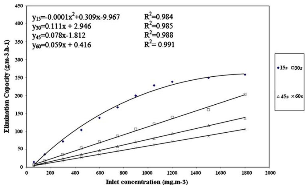
concentration of  $1 \text{ g m}^{-3}$  was suitable. With 21% oxygen in air, 48% of RE for benzene concentration below  $1 \text{ g m}^{-3}$  was achieved. The EC of bioreactor at pure oxygen injection condition was increased to  $386 \text{ g m}^{-3} \text{ h}^{-1}$ .
