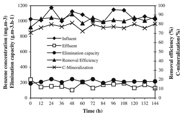
**Fig. 7** Continuous operation of bioreactor. Operation conditions: 6% *n*-hexadecane as organic phase, 0.2% Triton X-100 as surfactant, residence time of 15 s, biomass concentration of  $10\text{--}15 \text{ g L}^{-1}$ , The oxygen content in inlet air of 40%. C-mineralization is the percent of  $\text{C-CO}_2/\text{C-benzene degraded}$
