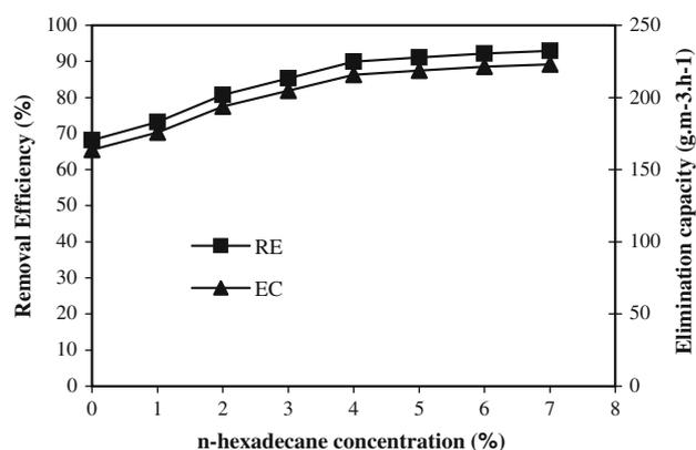
**Fig. 2** Effect of organic phase concentration on the bioreactor elimination capacity and removal efficiency for benzene. Experimental condition was:  $1 \text{ g m}^{-3}$  of inlet benzene concentration, 15 s of residence time,  $10 \text{ g L}^{-1}$  of biomass concentration
