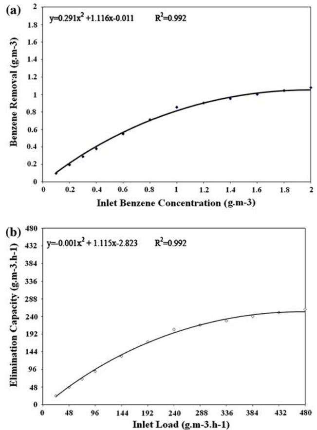
**Fig. 9** Trend of removal efficiency and elimination capacity of bioreactor for various inlet concentrations (a) and loads (b). Experimental conditions: residence time of 15 s and 10 g L<sup>-1</sup> of biomass concentration. Oxygen content was 40%
