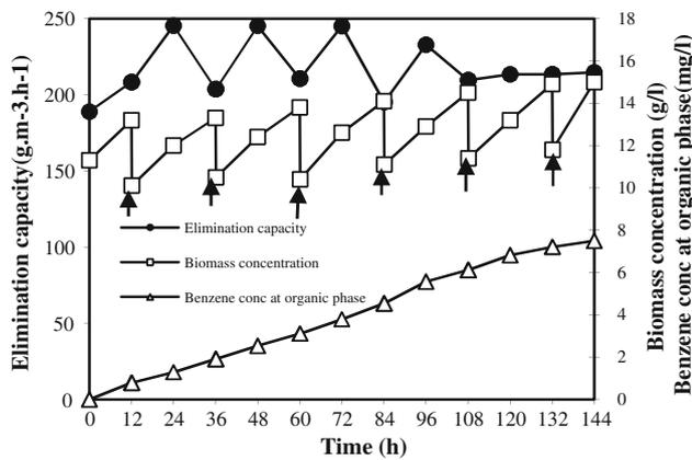
**Fig. 8** Changes of the elimination capacity, biomass concentration and benzene concentration in the liquid phase in continuous operation of bioreactor. The arrow indicates feeding of nutrient medium to bioreactor. Condition is similar to Fig. 5
