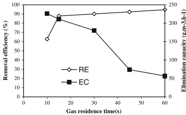
**Fig. 3** Effect of gas retention time on the bioreactor elimination capacity and removal efficiency for benzene. Experimental condition was: 1 g m<sup>-3</sup> of inlet benzene concentration, oxygen content of 40%, and 10 g L<sup>-1</sup> of biomass concentration
