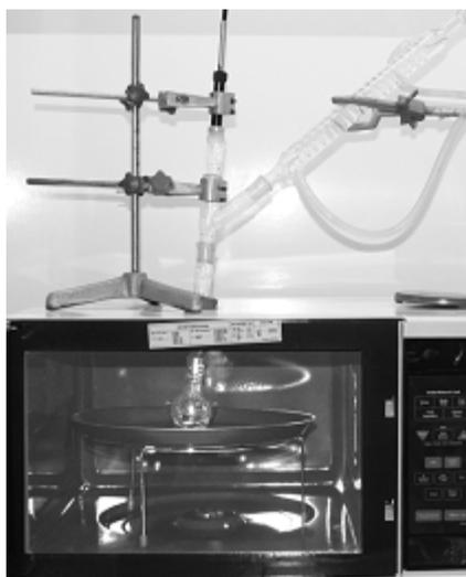
Figure 1. Assembly of the MA-HS-SPME
