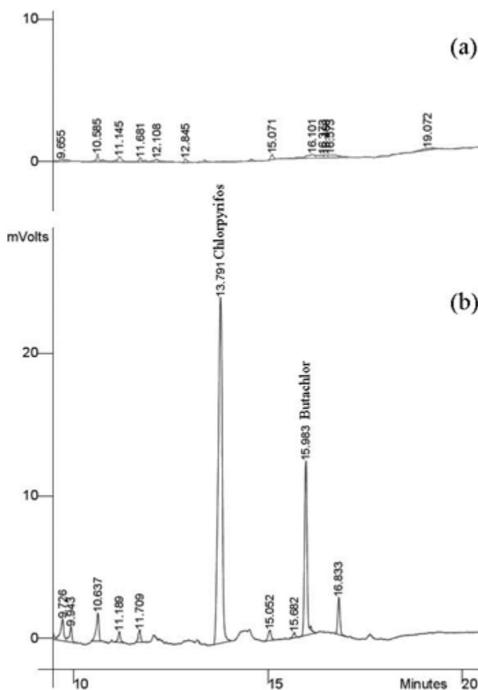
**Figure 4.** Chromatograms of urine sample (a) without and (b) with spiked sample of chlorpyrifos and butachlor
