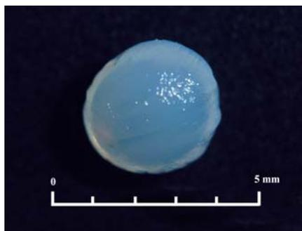
Fig. 1: Size and physical shape of chitosan bead
