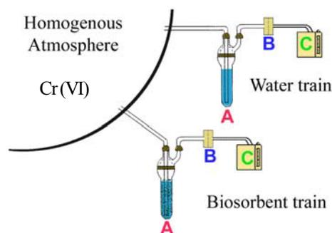
Fig. 2: Set up of the sampling trains
