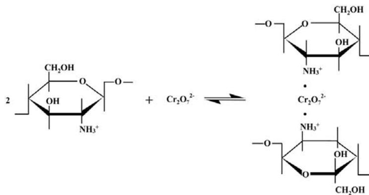
Fig. 5: Interaction between  $\text{NH}_3^+$  functional groups in chitosan and  $\text{Cr}_2\text{O}_7^{2-}$
