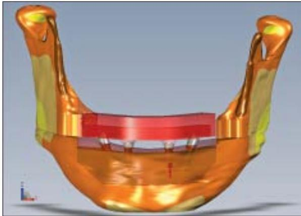
**Fig 1** Three-dimensional FE model of human mandible incorporating four dental implants supporting a one-piece superstructure. The posterior implants are tilted distally in the so-called All-on-Four configuration.
