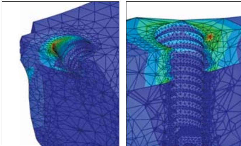
**Fig 4** Von Mises stress distribution in a buccolingual cross section of peri-implant (no. 1) bone during posterior loading. (Left) Model A; (right) model S. The color range from blue to red indicates stress or strain concentration from low to high.
