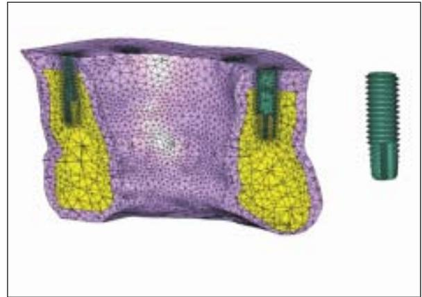
**Fig 2** Views of the meshed models. (Left) Peri-implant bone; (right) Nobel Biocare implant.
