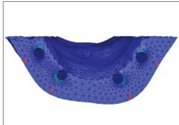
**Fig 3** Stress distribution in the peri-implant bone of model A during anterior loading. The color range from blue to red indicates stress or strain concentration from low to high.
