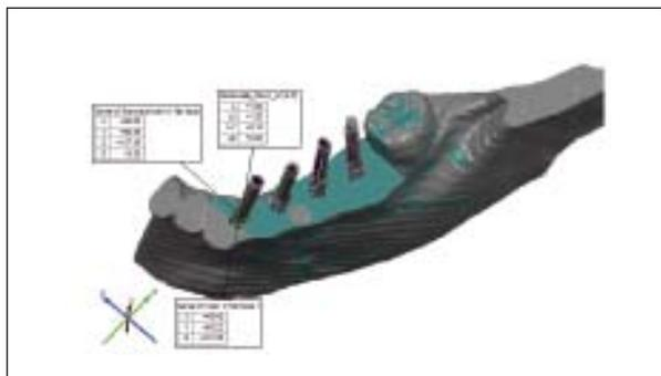
**Fig 11** Superimposition of the computerized models of the osteotomized jaw on the CAD data and calculation of differences in mesiodistal and buccolingual directions.
