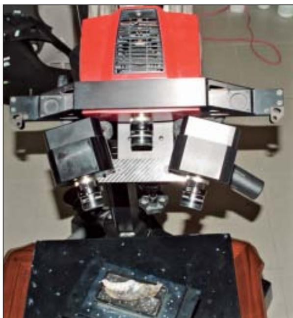
**Fig 6** Digitizing the nonanatomic template with the optical measuring technique (ATOSII).
