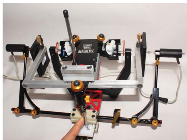
Fig. 2: The excursive movements were made manually up to 11 mm of the translation
