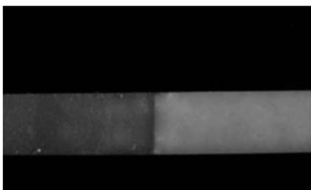
**Figure 1** Stereomicroscope image ( $40\times$  magnification) of a sound microbar ready for microtensile test.
