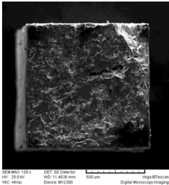
**Figure 2** SEM image (100× magnification) of a cohesive failure in veneering porcelain. Fracture originated and propagated in the veneer ceramic.
