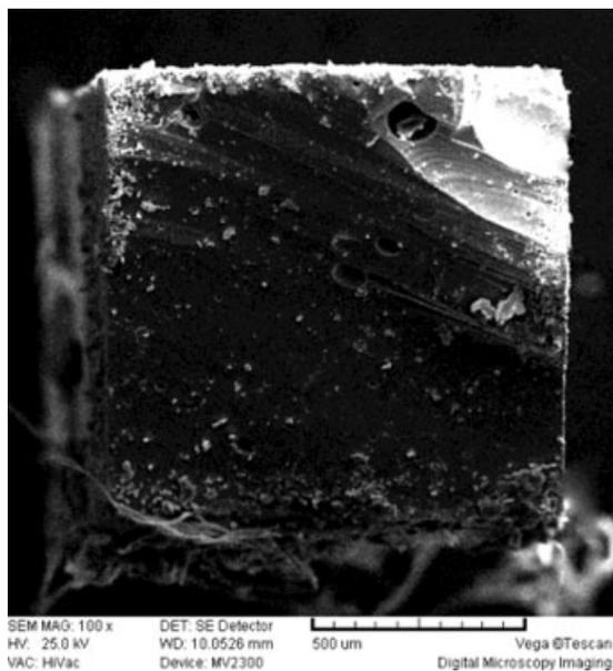
**Figure 3** SEM image (100× magnification) of a mixed failure. Fracture originated at zirconia/veneer interface, leaving exposed zirconia grains.
