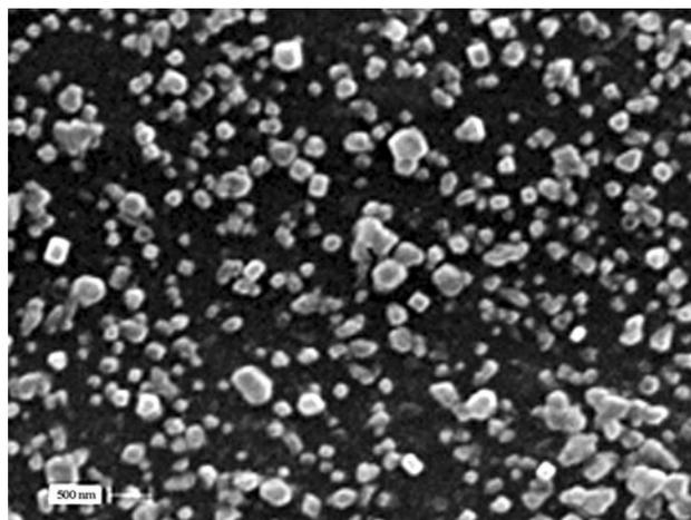
**Fig. 1** SEM image of the nisin-loaded chitosan/alginate nanoparticles
