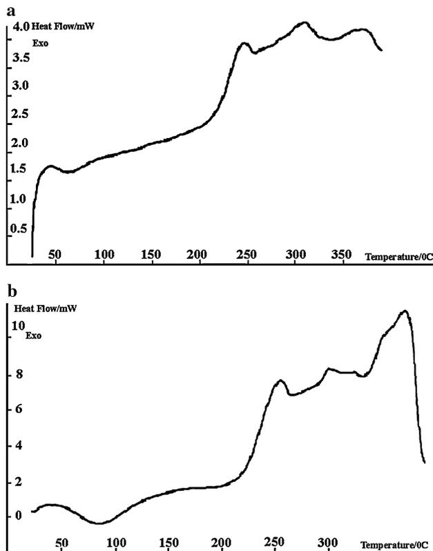
**Fig. 4** DSC thermograms of the chitosan /alginate nanoparticles and the nisin-loaded chitosan/alginate: **a** the chitosan/alginate nanoparticles; **b** the nisin-loaded chitosan/alginate nanoparticles
