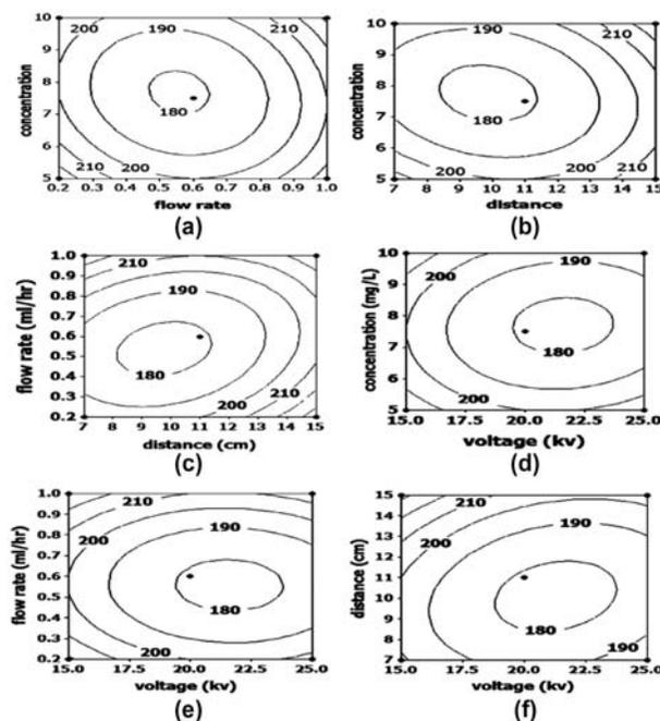
Figure 2. Counter plots of the response variable (fiber diameter (nm)) for the different experimental factors (two-factor-at-a-time). (a) Flow rate and polymer solution concentration, (b) distance and polymer solution concentration, (c) flow rate and distance, (d) polymer solution concentration and applied voltage, (e) flow rate and applied voltage, and (f) distance and applied voltage.
