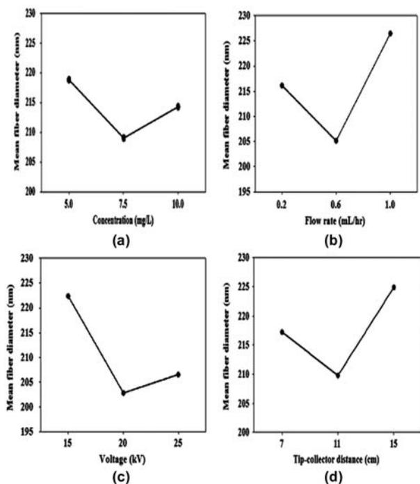
Figure 1. Effect of concentration, flow rate, voltage, and distance on the diameter of electrospun fibers.
