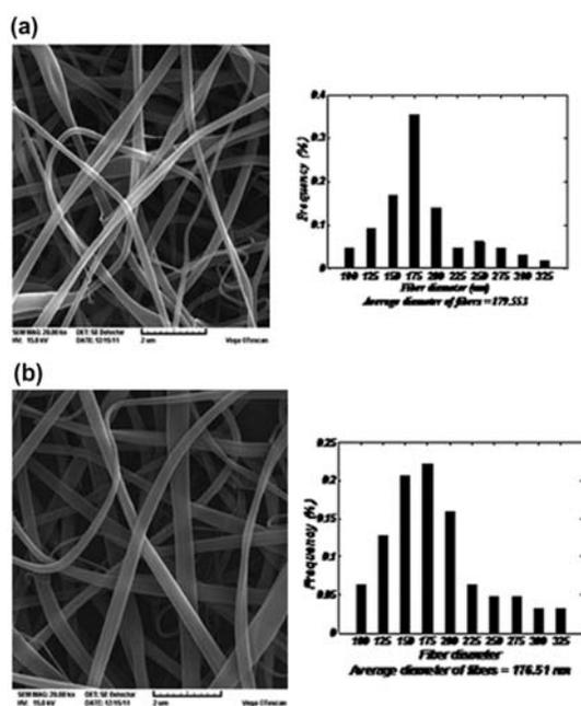
Figure 3. The SEM graphs of fiber scaffolds before (a) and after (b) optimization of electrospinning process.
