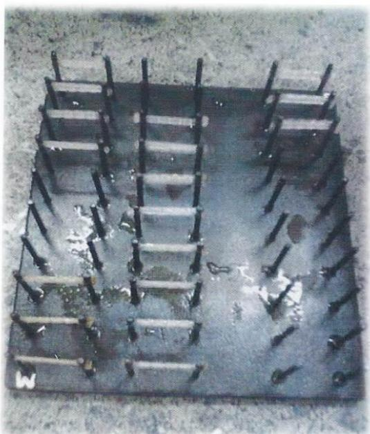
**Fig 1.** Custom made device comprising six rows of 40 pairs of pins which kept the elastomers stretched at the length of 25mm
