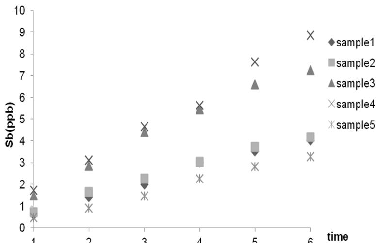
**Figure 2** Sb average concentration changes during storage (65°C).
