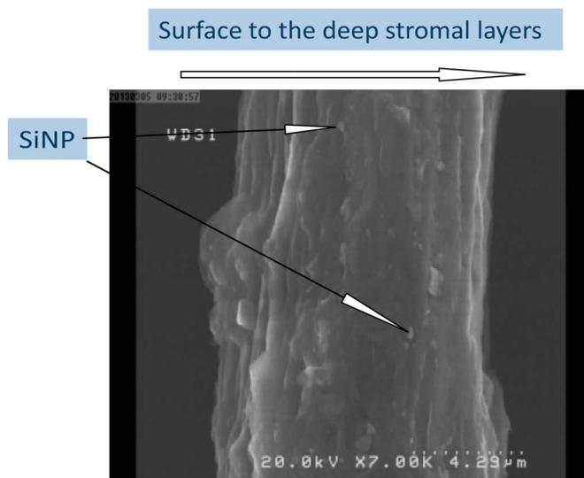
**FIGURE 4.** Transmission of SiNPs through the corneal stroma after 15 minutes by SEM: frozen section of vertical cut of the deep corneal stroma showing penetration of SiNPs of 40 nm.
