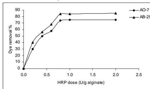
Fig. 7: Effect of immobilized HRP dose on dye removal. Conditions: dye concentration, 500 ADMI; enzyme concentrations, 0-2 units/g alginate; H<sub>2</sub>O<sub>2</sub>, 0.8 mmol/l; buffer phosphate, (pH=7.4); reaction time, 90 min at 25°C.
