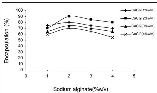
Fig. 1: Encapsulation efficiency, under different gelation condition, T= 25°C
