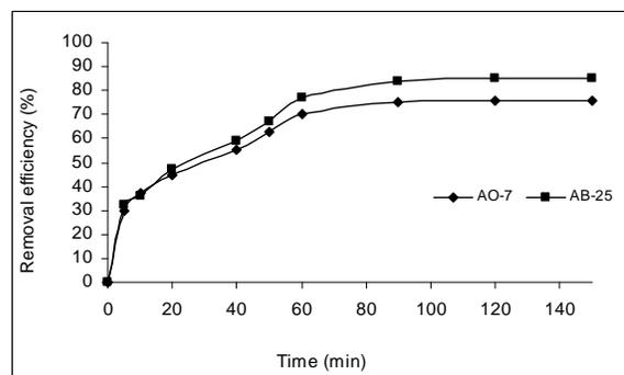
Fig.6: Effect of reaction time on dye removal by immobilized HRP. Conditions: dye concentration, 500 ADMI; enzyme concentration, 1 units/g alginate; 0.8 mmol/l, H<sub>2</sub>O<sub>2</sub>; buffer phosphate, (pH=7.4); reaction time, 90 min at 25 °C.
