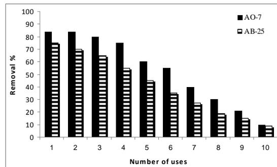
Fig.5: Reusability of capsules (cycles), Conditions: AO-7 and AB-25 concentrations, 500 ADMI; enzyme concentration, 1 units/g alginate; 0.8 mmol/l, H<sub>2</sub>O<sub>2</sub>; buffer phosphate, (pH=7.4); reaction time, 90 min at 25 °C.
